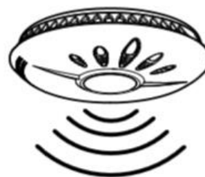
B) The unit will emit a loud (85dB at 3 meters) alarm for around 5 seconds and stop automatically.
